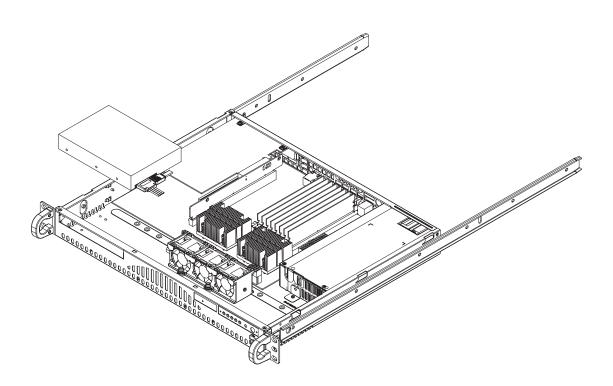
Figure 6-3. Removing the SATA Drive (with CD-ROM drive removed)
